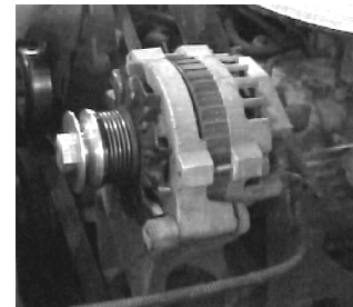
Add-A-Pulley™ attached to existing alternator.
