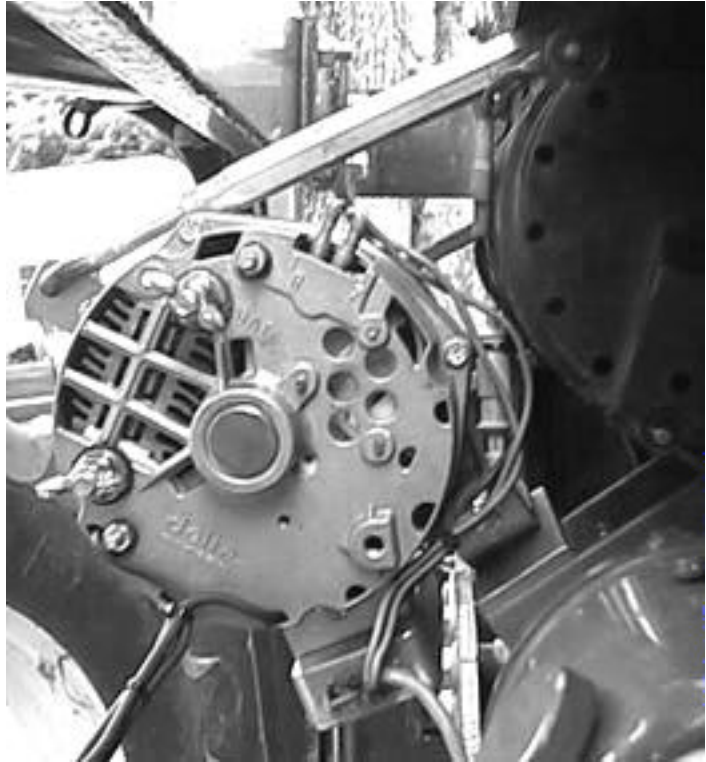
A Universal Mounting Bracket was used to mount the Power Generator to a fabricated bracket assembly
